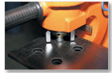
When selecting your tool, please note: For material DIN S233: maximum material thickness = 0.8 x hole Ø
