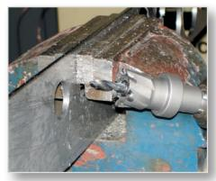
Free-hand drilling up to Ø 30 mm
