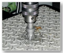
Drilling structured sheet metals
