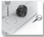
If the workpiece is especially thick ... ... it is also recommended that you cut from both sides, or drill a number of
